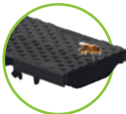
COMBee-design grating Ø 7,3 mm, cl. C plastic PA6 for NW 100
