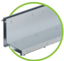
Slot top SW 12,5 mm, cl. B for NW 100 - galvanised steel, cl. C for NW 100 and 150 - galvanised or stainless steel
