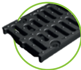
Ductile iron grating SW 15/75 - cl. F, 4 point bolted grating, for NW 150
