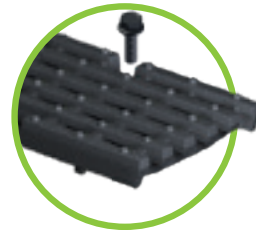
Ductile iron elongated bar grating, MW 22/13, cl. E, 4-point bolting only available in cast iron edge, for NW 100 to 200
