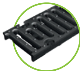
Ductile iron grating SW 16/120 or 16/220, cl. F - 4 point bolted grating, for NW 100 and 200
