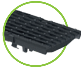
Ductile iron elongated bar grating, MW 28/9, cl. D for NW 100 and 150
