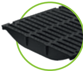
Ductile iron grating SW 20/170 - cl. F 4 point bolted grating, for NW 500
